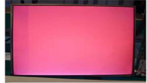
Vertical Block Source TAB IC Defect
