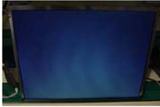
Panel Mura, Light leakage
