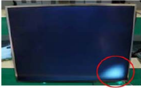
Panel Mura, Light leakage
