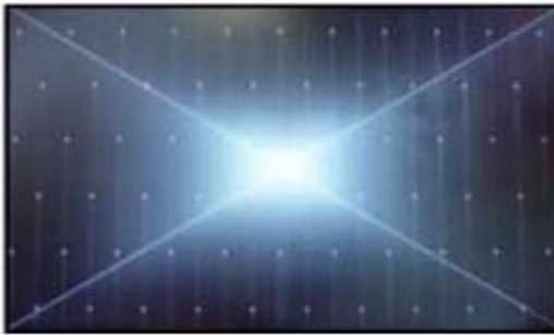
Solder defect, Short/Crack
