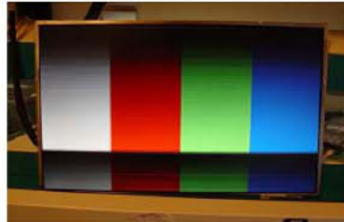
Horizontal Block Gate TAB IC Defect
