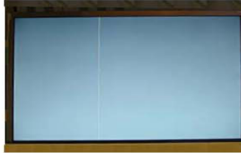
Vertical Line Source TAB IC Defect
