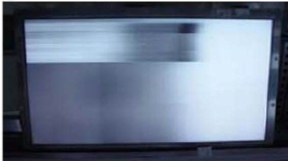
Horizontal Block Gate TAB IC Defect
